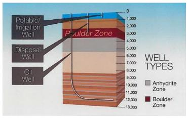
be inferred that, because oil is confined to the Sunniland reservoir, pathways for vertical migration of fluids (fissures or faults) do not exist.
