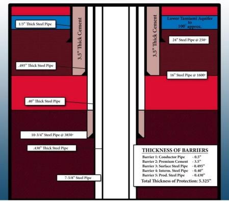
aquifer, a series of four, vertical, separate, protective steel casings and 3 feet 5 inches of cement surround all oil-producing wells in the region providing a 5-inch barrier between the aquifer and the oil being pumped to the surface.
