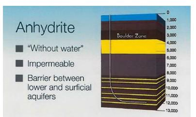
units, and vary in thickness from several hundred feet to more than a thousand feet. Under these conditions, it is not possible for the limited volume of fluids that may be injected during a stimulation procedure in to the oil bearing formation to "bubble up" through the multiple layers of impermeable formations.
